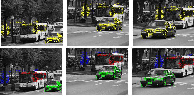
Figure 5: Motion segmentation: given feature points on multiple rigidly moving objects tracked in multiple frames of a video (top), the goal is to separate the feature trajectories according to the moving objects (bottom).
