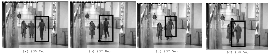
Fig. 11. Weakness of the method. The tracker fails and changes of target during the sequence because the new target has a higher classifier score then the initial one.
