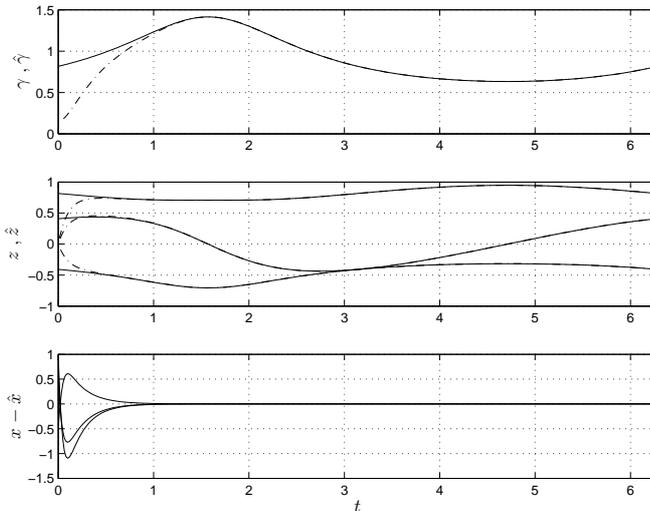
**Fig. 2.** Structure estimation results, using a circular camera motion. True (solid) and estimated (dash-dotted) values of  $\gamma$  (top) and  $z$  (middle). Estimation error for  $x$  (bottom).
