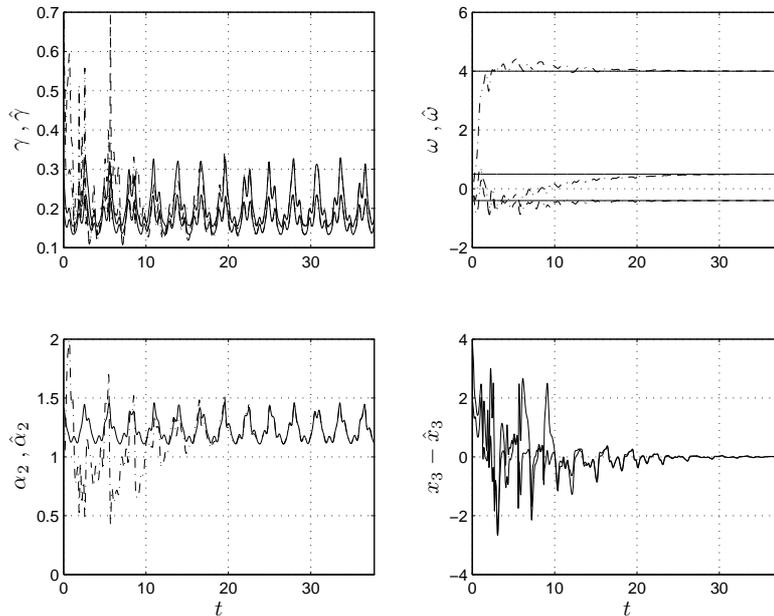
**Fig. 3.** Structure and motion estimation results, for a periodic object motion as in [23]. True (solid) and estimated (dash-dotted) values of  $\gamma$  (upper left),  $\alpha^2$  (lower left) and  $\omega$  (upper right). The depth errors are shown in the lower right plot.
