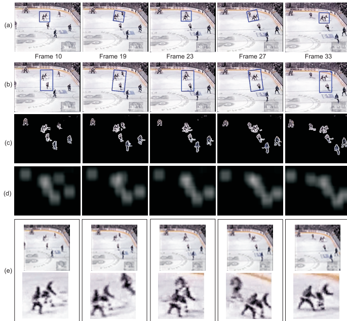
Fig. 5. Ice hockey game example. (a) The input key-frames with the computed active windows highlighted in blue. (b) Using a different size, our method can also produce an optimal output highlighted in blue. (c) The extracted foreground pixels. (d) The corresponding density map. (e) A comparison with the results from directly resized video and our approach.
